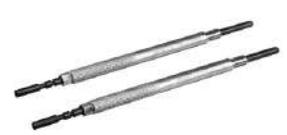
FERR.P/ POSICIONAR PISTOES PALIO 1.0/1.3/16V
